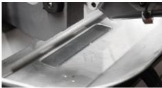
A large, easily accessible chip tray with dripping An adjustable guide cube provides the possibilisieve prevents the coolant from flowing out the ty to be set as close to the material as possible. machine.
