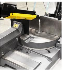
A lever for fast-feed control is located ergonomically on the left side of the vice.
