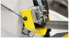
The saw blade guidance is enabled by ground hard metal elements of cemented carbide, always providing the greatest accuracy of the cut
