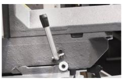
Vice fast-feed ability provides a possibility of quick re-adjustment of clamping jaws according to the size of material in just a few seconds.
